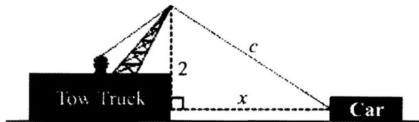
A car is attached to the winch on a tow truck by a steel cable. The top of the cable is 2 metres above the point of attachment. At time  $t$  seconds the length of the cable is  $c$  metres and the winch is reducing this at the rate of  $\frac{dc}{dt} = -0.1$  m/s. The horizontal distance between the car and the tow truck is  $x$  metres. The situation is shown in the schematic diagram above.
